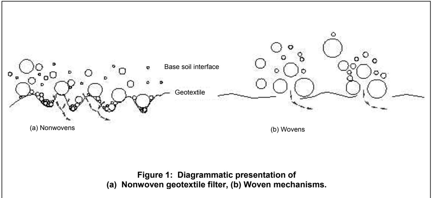
However, for the same base soils there is often a question as to whether a non-woven or woven geotextile could or should be used *in unidirectional flow applications*.
